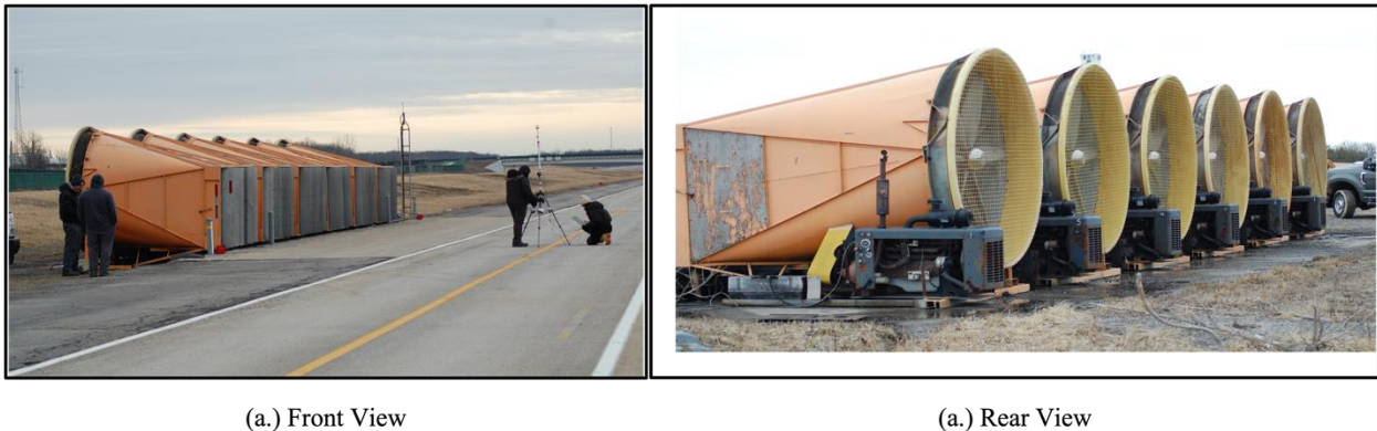
Figure 2-18. Front and rear view of the crosswind fan array at the Skid-Pad Facility located at the Transportation Research Center (TRC).
