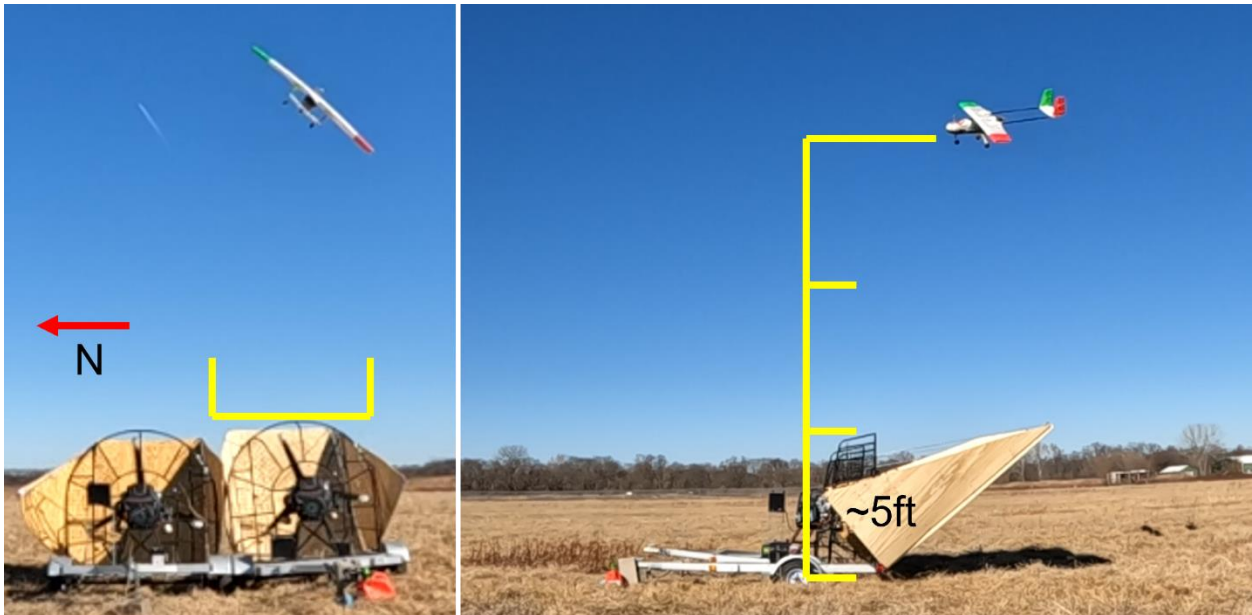
Figure 3-61. UAS Headwind Encounter: South fan @ 60%, North @100%, 11 ft above fans, 3 ft laterally.
