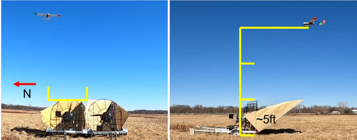
Figure 3-60. UAS Headwind Encounter: South fan @ 60%, North @100%, 11 ft above fans, 5 ft laterally.
