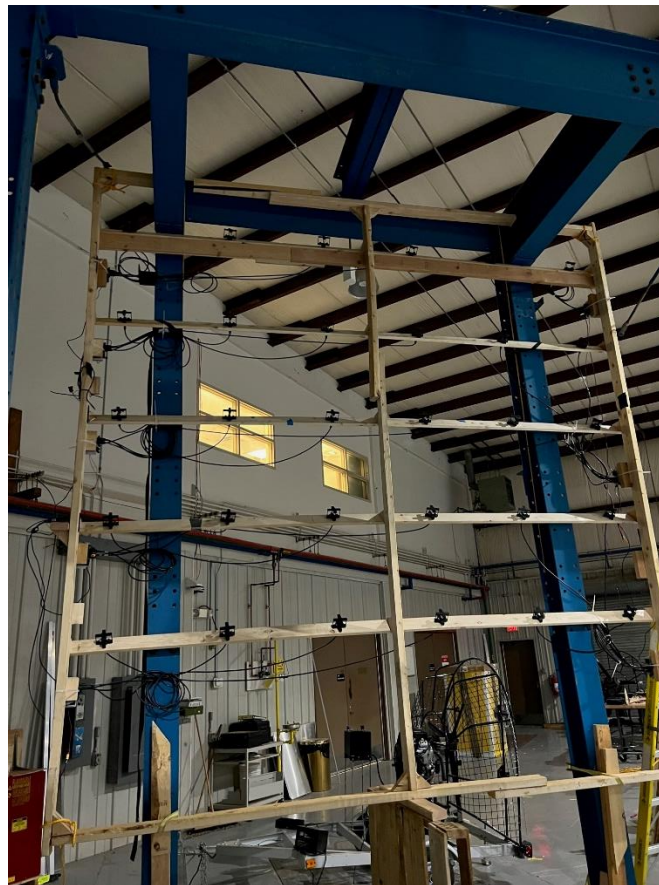
Figure 2-14. 30-channel TriSonica anemometer array in a vertical orientation.
