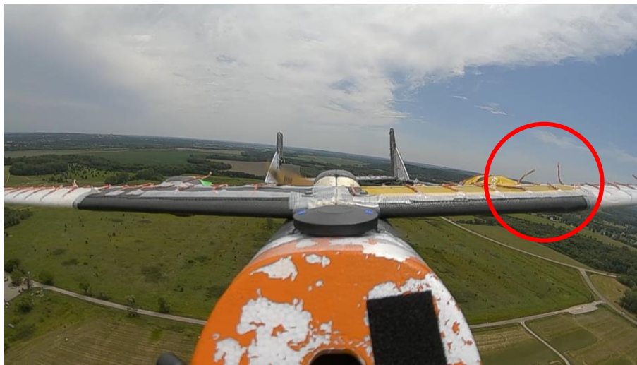
Figure 3-53. Tufts during unstable flight.
