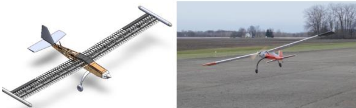
Figure 5-1. Flutter Flight Test Vehicle CAD rendering (left), and flying (right).
