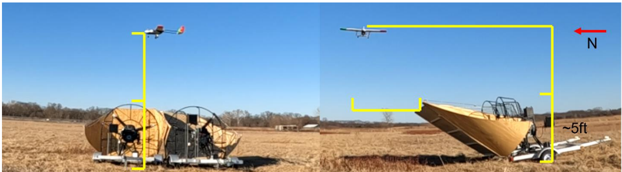
Figure 3-62. UAS Side Encounter, Both Fans at 100%, 5 ft above fans, 5 ft laterally.
