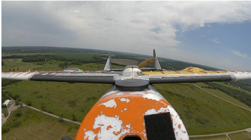
Figure 3-52. Tufts during stable flight.
