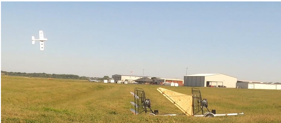
Figure 3-56. AeroScout upset by fans (fan on left with early air flow deflection “paddles”).
