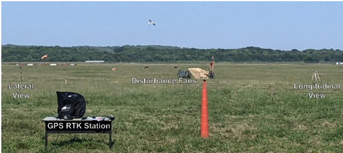
Figure 3-55. Flight test ground support around fans: ground station and two cameras with different views.
