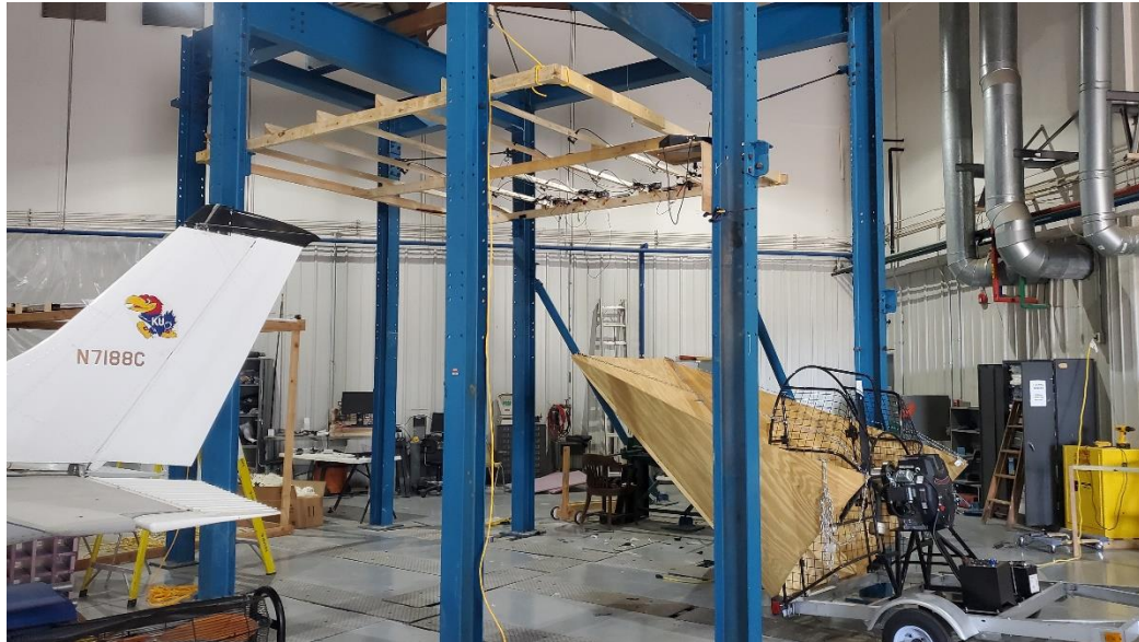
Figure 2-12. Anemometer array positioned horizontally to measure wind machine output.
