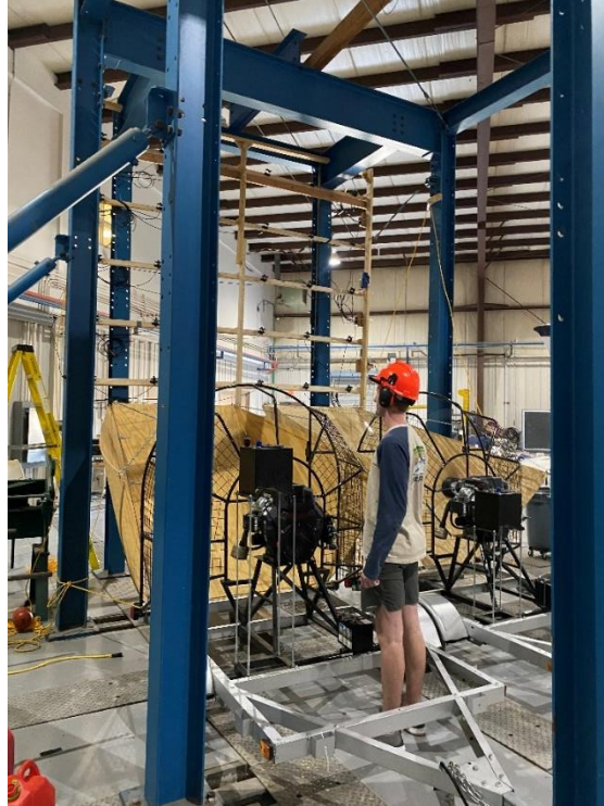
Figure 2-15. Two fans side-by-side being characterized, positioned in front of an anemometer array.
