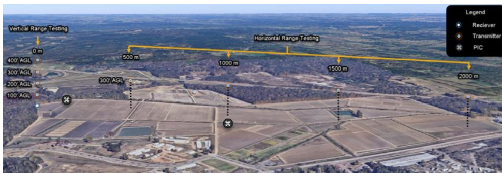
Figure 8. Test point locations for the preliminary range test.
