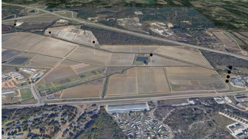
Figure 9. Test points for Parrot ANAFI Wi-Fi beacon and Dronetag range testing.
