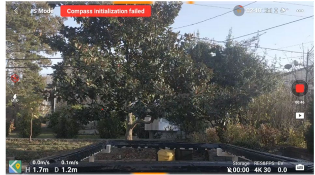
(d) Onboard video recording with the compass failure warning at near position with 2.2-kA excitation
