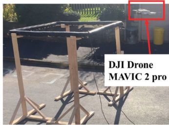
(a) Exhaustive test of UAS on top of planar coil
