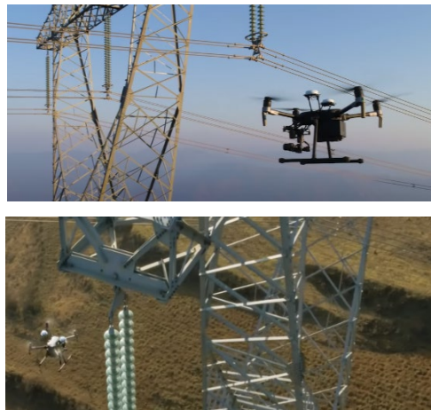
Figure B5. Drones in close proximity to transmission lines for inspection (DJI 2017a).
