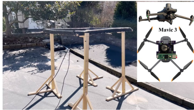
Figure 2-48. Experimental setup of Mavic 3 with a sensor board payload testing in 2.2-kA planar coil environment that can generate 60 Hz ac magnetic field.
