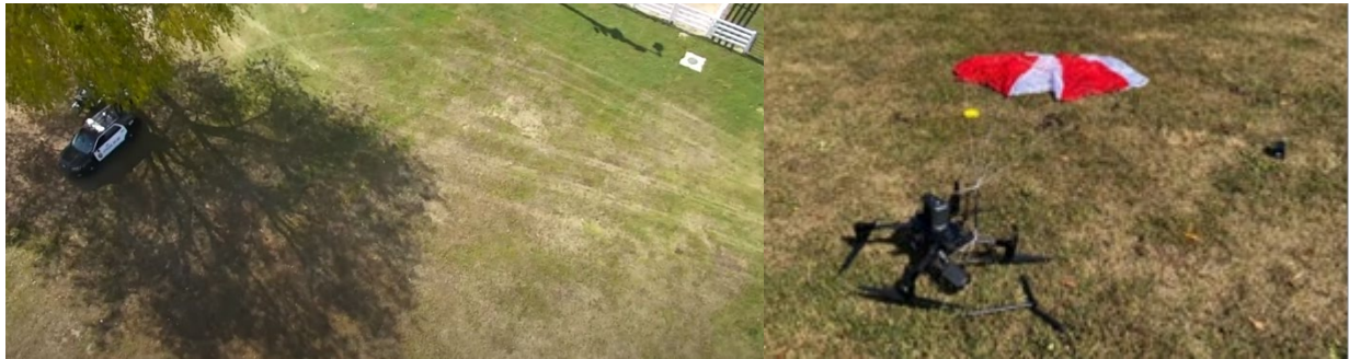
Figure B9. Third party drone parachute system ParaZero erroneously deploys. Last frame that was captured from the video feed (left) before the crash (right) (Report Drone Accident 2020b).
