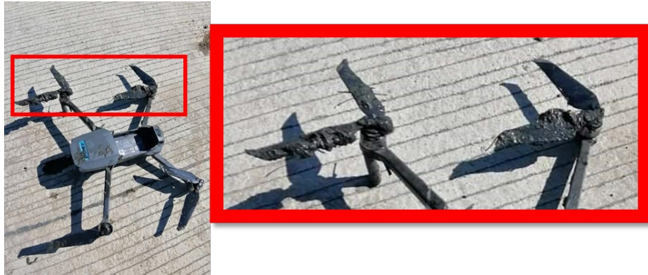
Figure B6. Drone damaged from physical contact with a powerline (Lee and Choi 2017).
