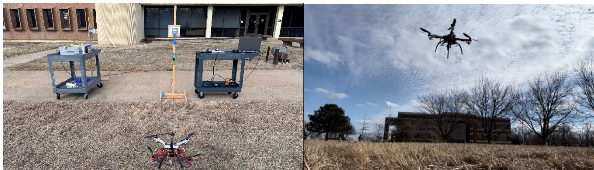
Figure 4-36. Front-door RFI flight tests. Left: setup (also compare to Figure 4-32). Right: QwinOut F450 model during flight
