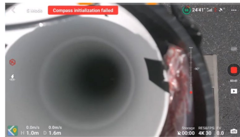
(d) Onboard video recording with the compass failure warning at near position with 7.5-kA excitation
